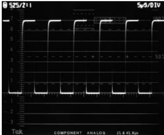
Figure 3b. Example of a square-wave calibration signal.
